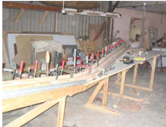
The problem with the Minimoa spars are they bend in two directions at the gull wing point. I determined that if I built a bent table with the bend equal to the sweepback of the spar, and offset the inner section of the spar off the centerline equal to the gull angle, I could then construct the spar caps in place on the front plywood webb of the spar, with the ply on the table top allowing me to clamp the laminates into place including the bends required.
